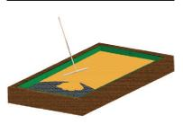
Cover the entire area with a 5-10mm bedding layer of sharp sand / soil mix and compact.
