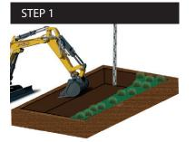
Excavate area for subbase to be installed. *For subbase calculation see overleaf.* Ensure to allow for: 10mm sand bedding layer; depth of grid and the 10-15mm dressing of aggregate when calculating depth from surrounding surfaces.
